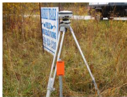
Sokkia GRX1 GNSS Receiver set over GCP 2
