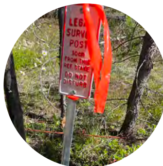
Example of a metal reference post
