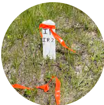
Example of a Wooden Guard Stake
